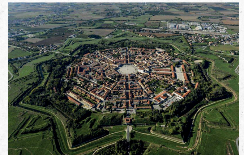
fig 2. Palmanova from above (Art Travel, 2014). A real life example of the Florence Star Shape city plan, structured to withstand canon fire, with an emphasis on a centralized military and religious community.
